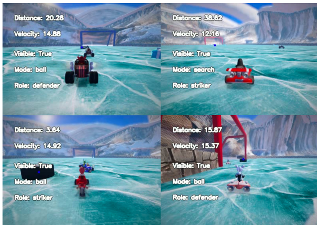
Figure 2. Sample vision network prediction. We observed that the system is able to accurately detect the puck visibility, aimpoint and distance for various player types and game combinations.
